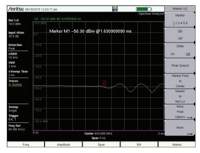
Figure 5. Audio Delay through a Motorola GR1225 analog repeater.
