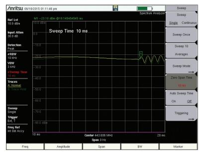
Figure 4. Delay through a Motorola Quantar with 10 MS trigger delay. Note the green trace is a reference and the yellow trace a second measurement with a 40 us audio delay to the speaker.
